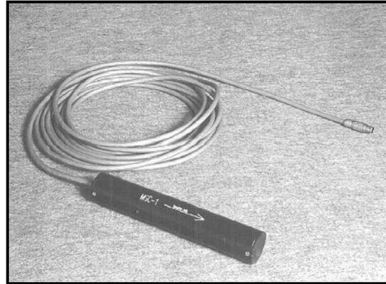
The **MGC-1** also includes a calibration winding that can be used to verify performance or perform a health check.
