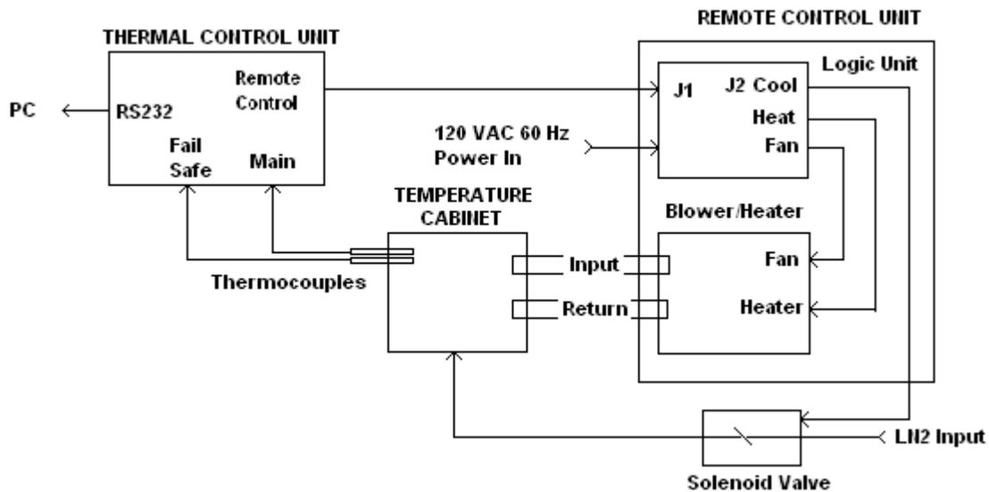
Figure 1 Thermal Control System configuration.
