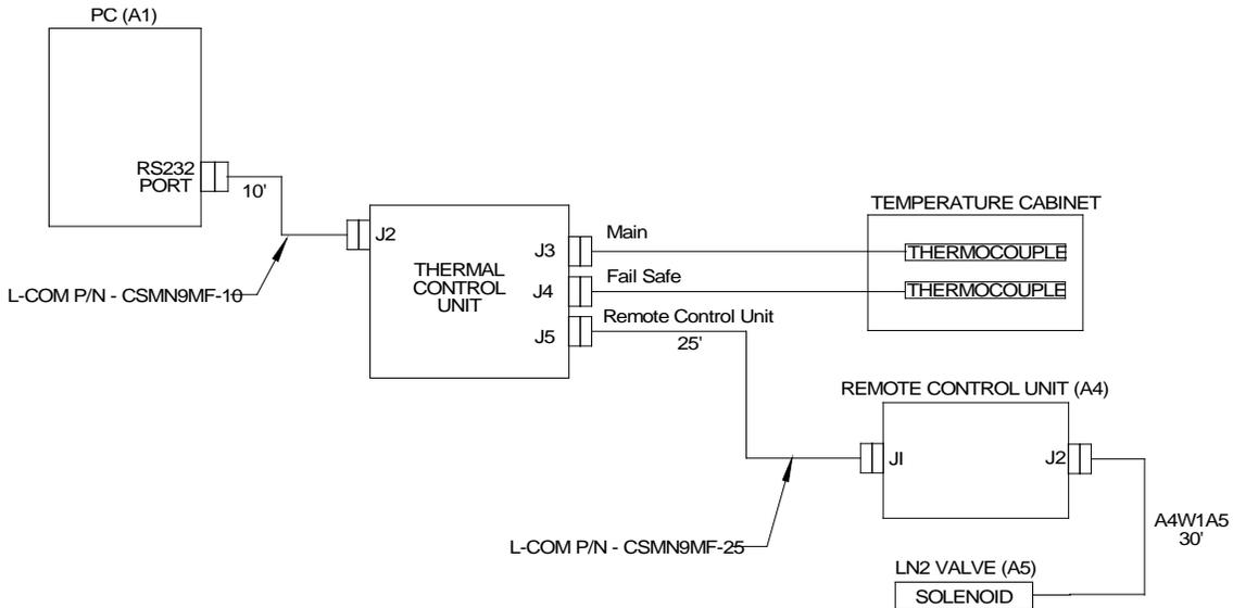
Figure 9 Thermal Control System Cabling
