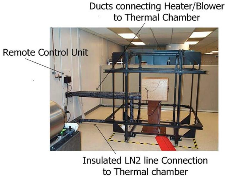
Figure 8 Typical Installation
