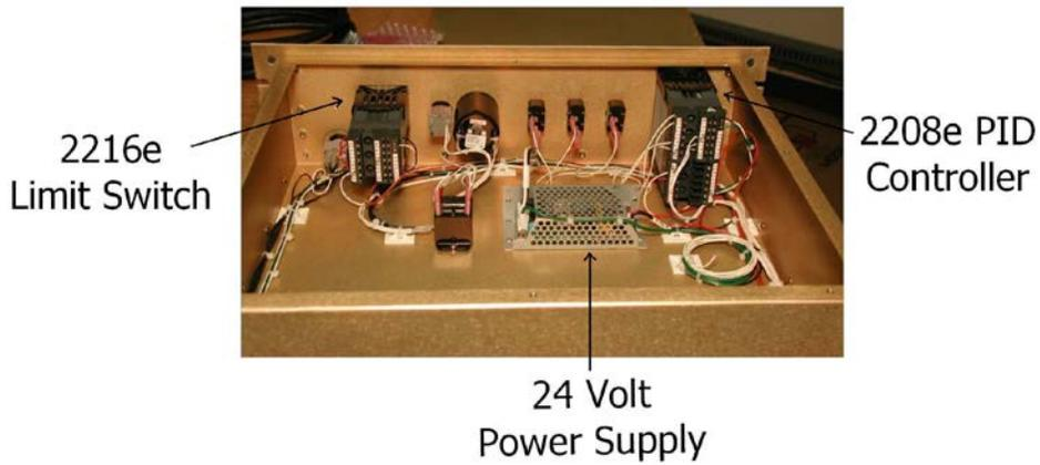
*Figure 4 Rear View of Controller Interior*
