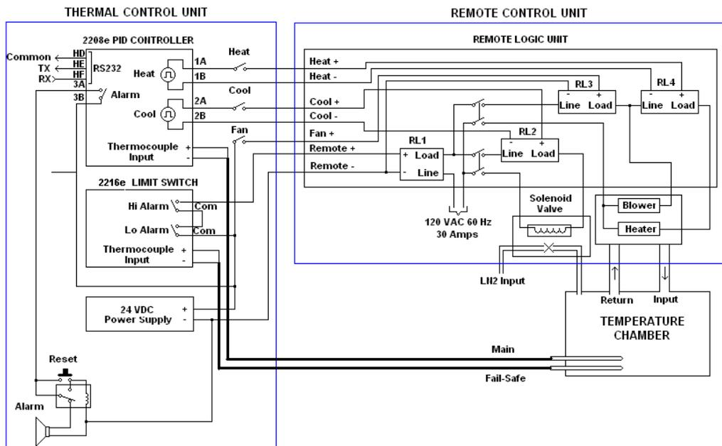
Figure 2 Thermal Control System functional block diagram
